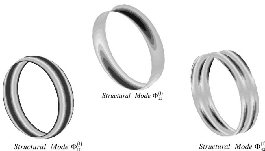
Fig. 2. Nodal patterns for circular cylindrical shells.
